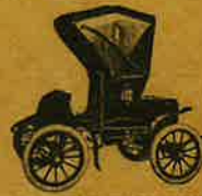
THE STUDEBAKER STANHOPE Single, 8 to 9 h.p., electric motor, motor of brass, 28 and 30 inch wheels, 27 inch wheelbase, 60 inches, 1700 lb. weight weight, 1250 pounds, 2000 lbs. weight, 2000 with top, $1,275.—Studebaker Bros., Co. of New York, New York.
